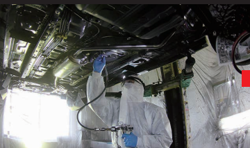
Remove undercarriage cover and spray "Black" (approx. 2 - 3 ℓ)
