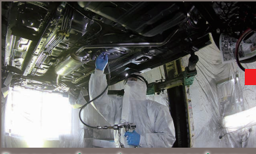
Remove undercarriage cover and spray "Black" (approx. 1.5 - 2 ℓ)
